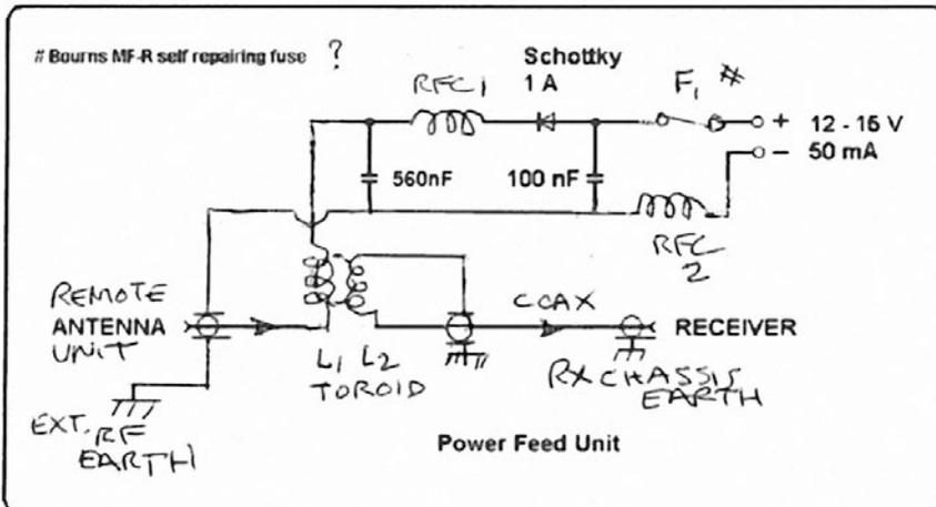
article in which he suggests making an earth connection via a back-back panel-mount BNC in series with the coax.
