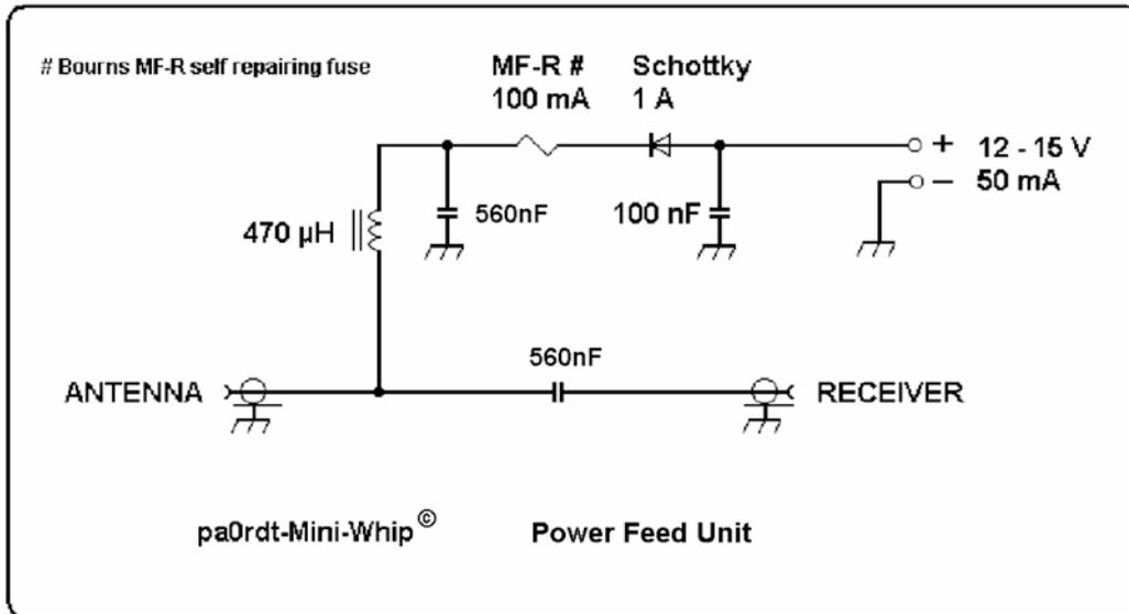
Power is fed to the **pa0rdt-Mini-Whip**® via the coaxial feed line. A Power Feed unit couples the power through the coaxial feed line to the **pa0rdt-Mini-Whip**®. A second coaxial cable couples the signal to the receiver.
