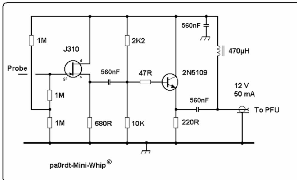
The circuit diagram of the RF section of the mini-whip which was previously shown in Part1 of this article is repeated again above to save referring back to the original.
