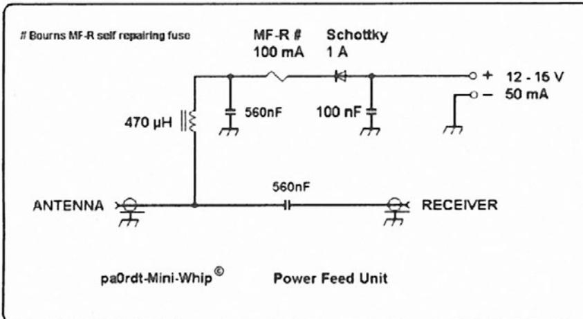
**Fig 3 Power Feed Unit circuit diagram.**
