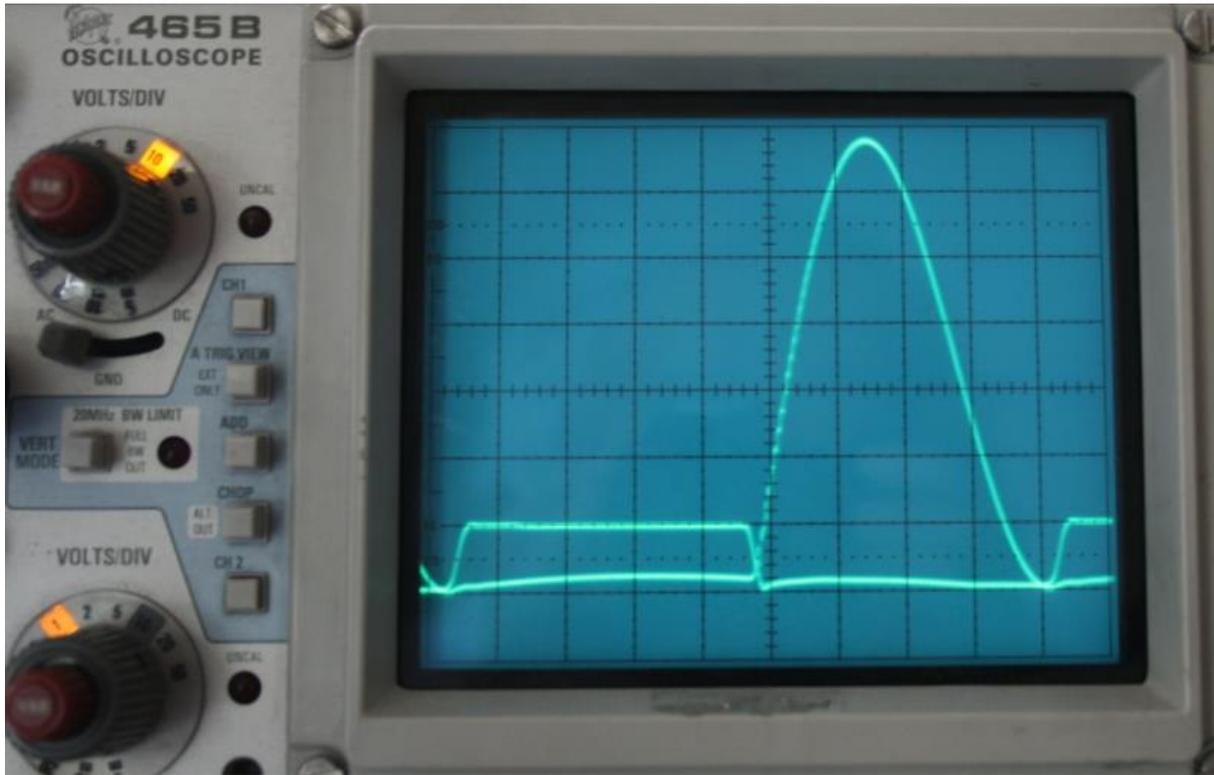
Figure 5 Gate and drain waveforms for properly adjusted class E PA (Both waveforms 10 V/div)
