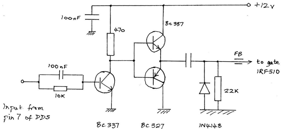
Figure 2 Driver stages for 472 kHz PA (Missing capacitor value is 100nF)
