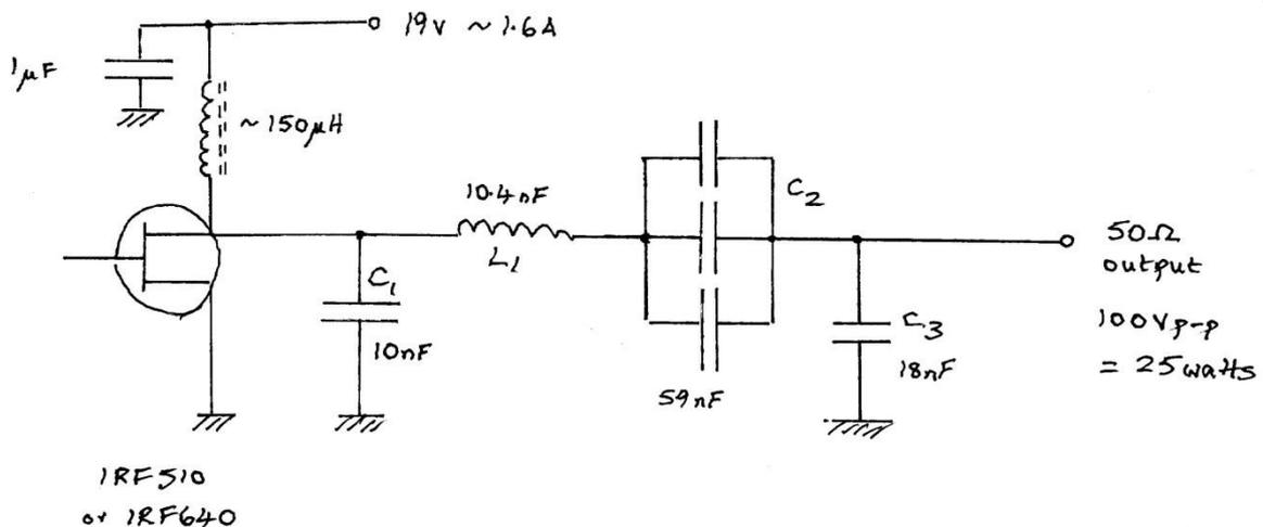
Figure 3 472 kHz PA stage
