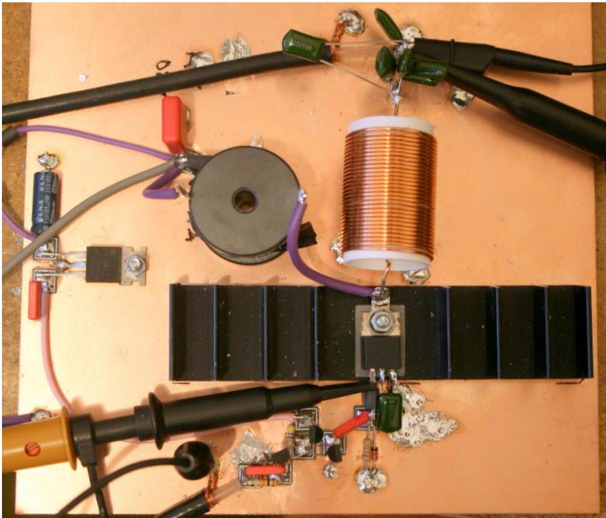
Figure 4 472k Hz driver and PA
